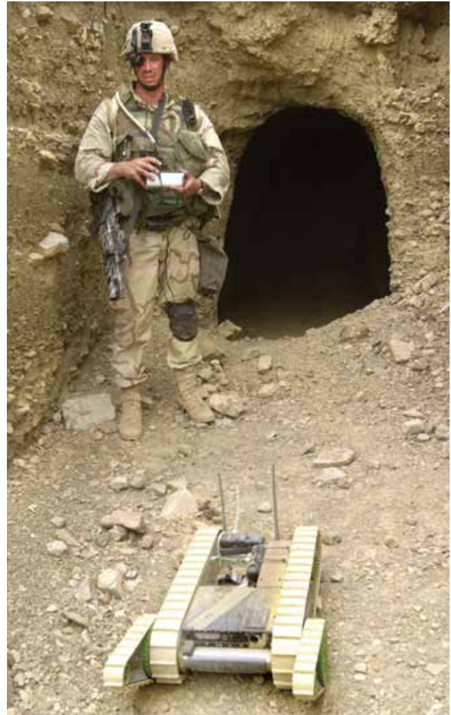
A U.S. army soldier manoeuvres “Hermes” the robot into a cave to detect mines, traps, and other unexploded ordnance. Photo: AP Photo/Wally Santana
